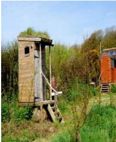
The composting toilet is a cheap alternative when mains toilets are not an option and when looked after and maintained properly can provide an environmentally friendly and odour free option. They work by turning human waste into an organic composting material which can safely be used to fertilise the soil, this happens using biological processes.
