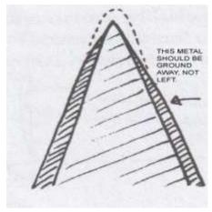
Do not rub files backwards and forwards as this blunts them: they cut on the forward stroke; sharpen away from the edge, steady the file end with your leather gloved hand. A file must be sharp - it cuts into the metal, not skids across it. Rub white chalk on it to stop particles accumulating; clean it with a wire brush, or push a wooden wedge along it. Files do wear out, so if yours is on skid row get a new one.
