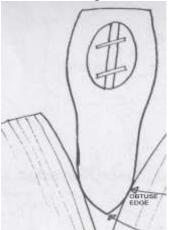
Sharpen an axe with a round stone. The stone has a medium and fine side, so start with the medium one - and grind with a circular motion, less than the width of the stone. Then finish off with the stones fine side. Take care to keep the convex, obtuse edge angle, and not to flatten that out.
