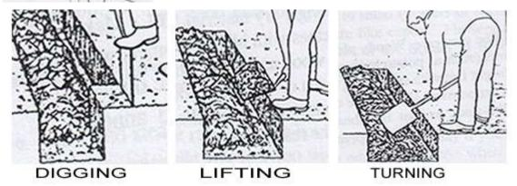
Digging is important. Try not to bring soil from the bottom of the trench to the surface, and do not use your spade as a lever nor crow-bar, or you will break it at the weld.
